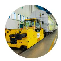
Electric shunter for internal rail maneuvers
