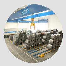
Two indoor 50 tonne bridge cranes and a fleet of custom forklifts for coils
